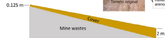
FIG 10 – Schematic diagram of cover system with increasing thickness from top to bottom of slope.
